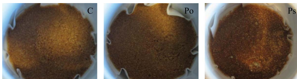
Fig. 4. Abiotic control (i.e. without fungus) (C) and fungal growth (Po: Pleurotus ostreatus ; Ps: Penicillium simplicissimum ) in contaminated cork after 61 days of incubation.
