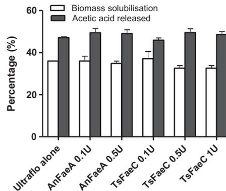
Fig. 3. Effect of feruloyl esterase supplementation to 450 U Ultraflo/g biomass on the solubilisation (white bar) and release of acetic acid (black bar) from whole Elephant grass after 96 h incubation at 37 °C.
