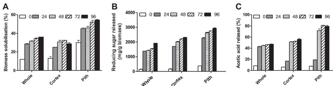
Fig. 1. The effect of Ultraflo on the (A) solubilisation, (B) release of reducing sugars, and (C) release of acetic acid from Elephant grass cortex and pith over a 96 h incubation at 37 °C.
