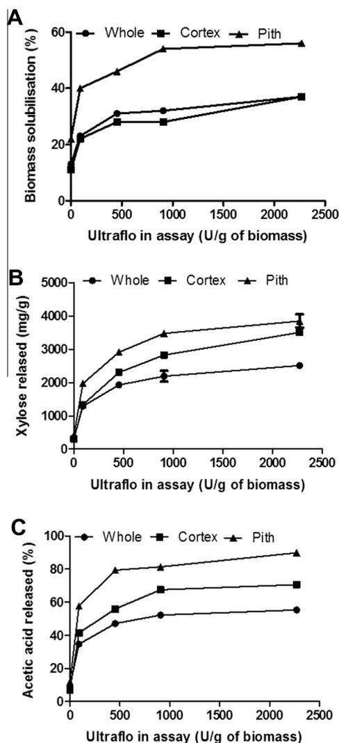
Fig. 2. The effect of Ultraflo dosage on the (A) solubilisation; (B) release of reducing sugar (expressed as xylose-equivalents); and (C) the release of acetate from whole Elephant grass (●), cortex (■) and pith (▲) after 96 h incubation at 37 °C.
