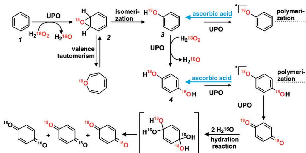
Figure 5. Scheme for the epoxidation/hydroxylation and further oxidation of benzene (1) and its following products phenol (3) and *p*-hydroquinone (4) by UPO via the benzene epoxide intermediate (2) (in the same way, catechol may be oxidized to *o*-benzoquinone). Adapted from Karich et al.<sup>57</sup>
